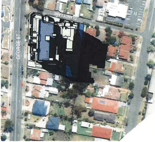
21ST JUNE 2PM - SHADOW DIAGRAM SCALE 1:1000
