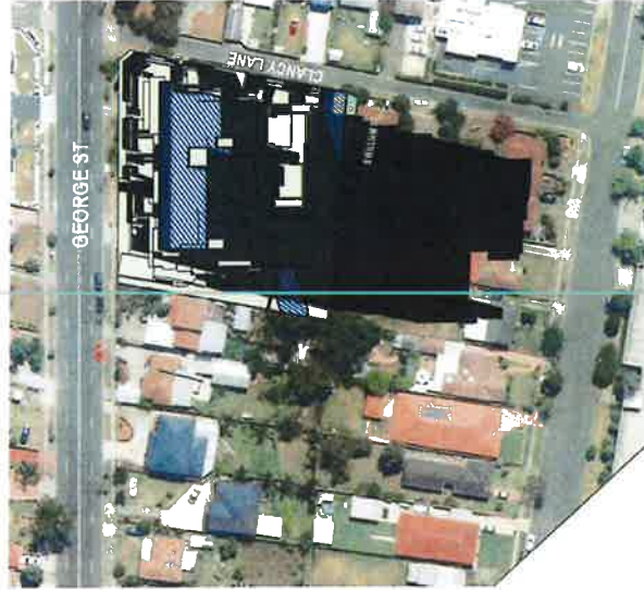
21ST JUNE 3PM - SHADOW DIAGRAM SCALE 1:1000
