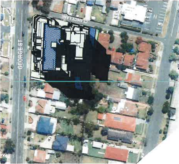
21ST JUNE 1PM - SHADOW DIAGRAM SCALE 1:1000
